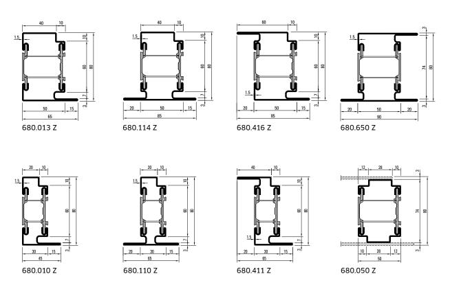
Z = made from hot-dip galvanised strip
