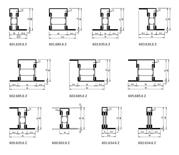
Z = made from hot-dip galvanised strip
